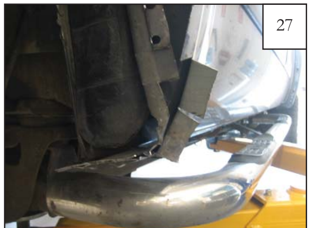
Bend remaining metal back even with other tabs. Note: Remove any additional overlap.
