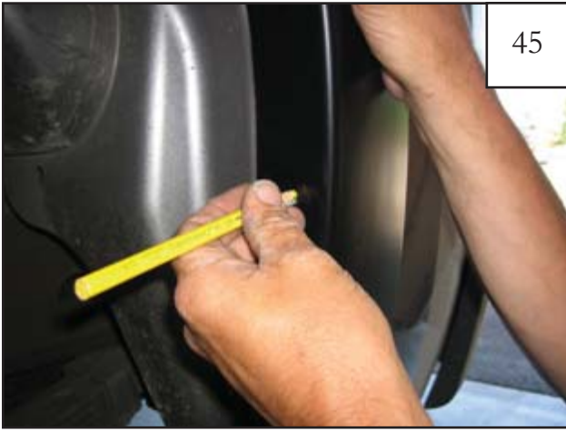
Holding flare in position on fender, use a grease pencil to mark eight hole locations.
