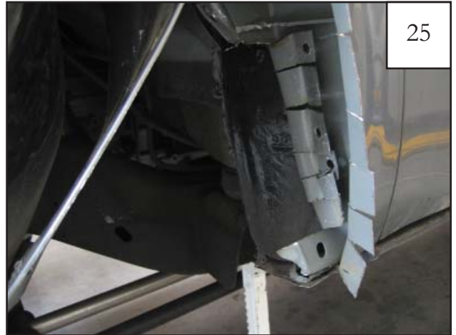
Inner flange flush against wheel well wall.
