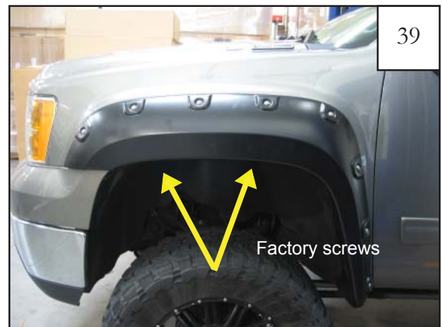
Using a 7mm socket reinstall two factory screws through flare, holes in splash shield, and into factory screw clips at top two locations.
