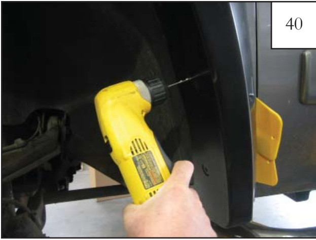
At two locations in the rearward side of the flare, drill through hole in flare and into sheet metal of vehicle.
