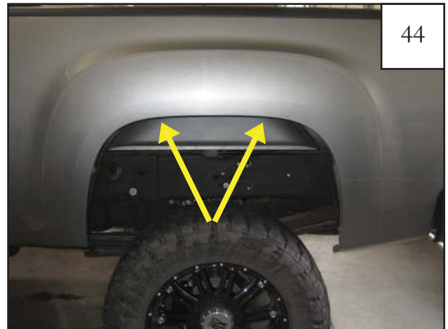
Tuffloc locations NOTE: If fender liner is installed. Remove factory tufflocs.
