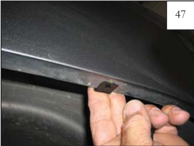
Center a supplied Clip (NU1-0007) over the marks made in Step 45. Clips may need to be adjusted to align with holes in flare. Note: The raised collar on the clip should face upward into the interior of the fender.
