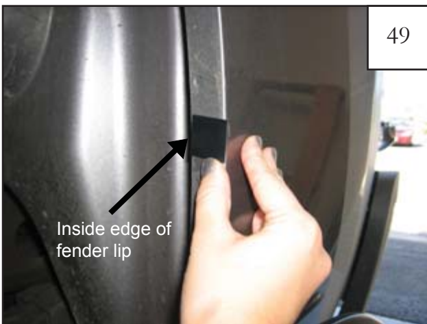
Center a supplied Tab (MT1-0002) over the six remaining marks made in Step 46, aligning edge of tab with inside edge of fender lip (tab may extend over outside of fender).
