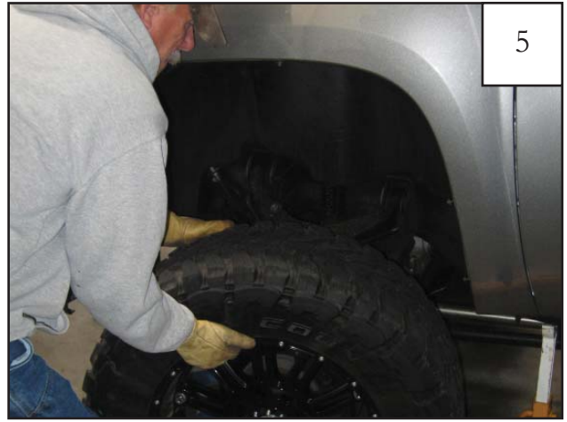
Support vehicle and remove tire.
