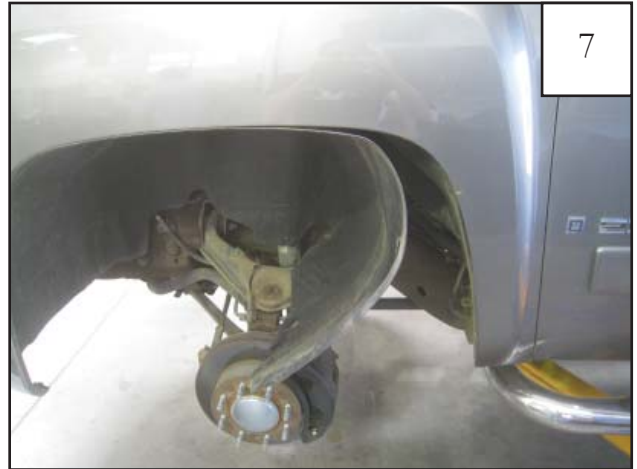
Pull back plastic shield and tie it to the axle with string or twine to keep it out of the way.
