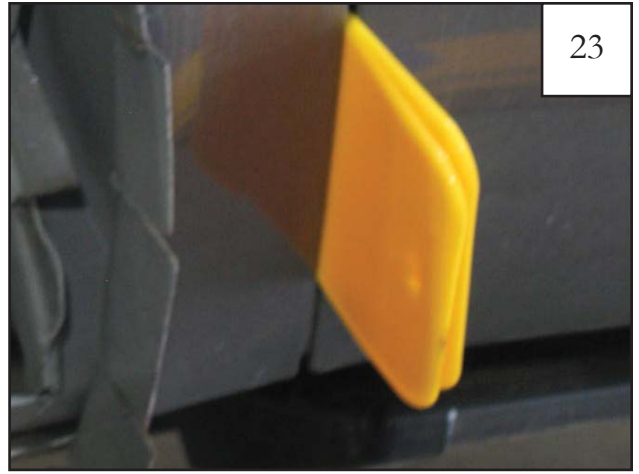
To prevent paint damage, insert body filler spreader or plastic spacer between fender and door. This will keep the fender from hitting the door edge while pounding back sheet metal in the next few steps.
