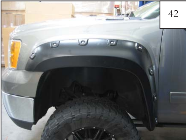
Reinstall wheel. Completed front flare installation.
