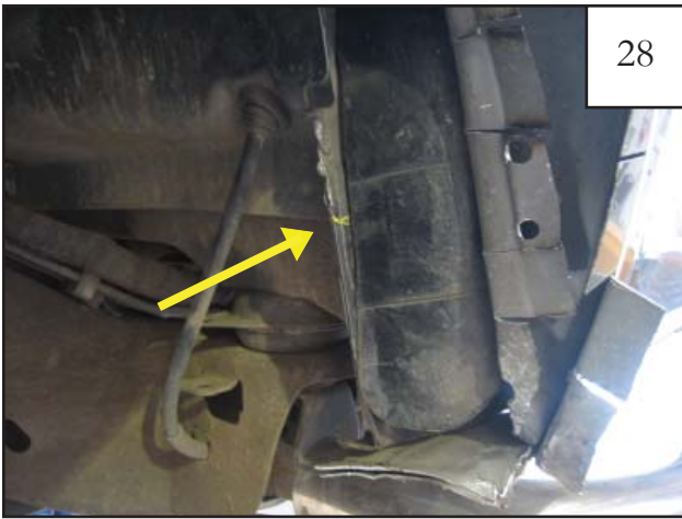
Mark inner pinch seam 8.25" from the bottom at location shown.
